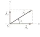
can represent any vector lying in the xy-plane as the sum of a vector parallel to the x-axis and a vector parallel to the y-axis. These two vectors are labeled  $\vec{A}_x$  and  $\vec{A}_y$  in the figure above (we will drop the use of arrow with boldface letters); they are called the component vectors of vector A, and their vector sum is equal to **A**.  $A = A_x + A_y$
