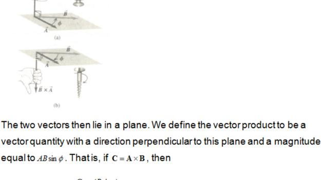
$C = AB \sin \phi$ We measure the angle  $\phi$  from A toward B and take it to be the smaller of the two possible angles, so  $\phi$  ranges from 0° to 180°. Thus C in the above
