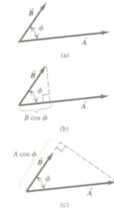
The angle between their directions is  $\phi$ ; the angle  $\phi$  always lies between 0° and 180°. The projection of the vector B onto the direction of A is the component of B parallel to A and is equal to  $B\cos\phi$ .
